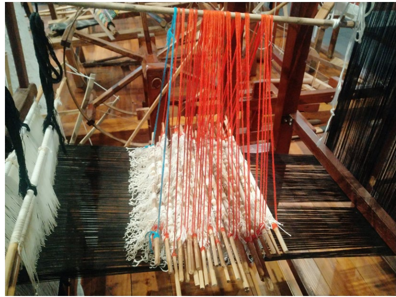
Fig 4. (left) Zhuang brocade loom from Jingxi in Guangxi Province; (right) Its multiple heddle pattern device.
