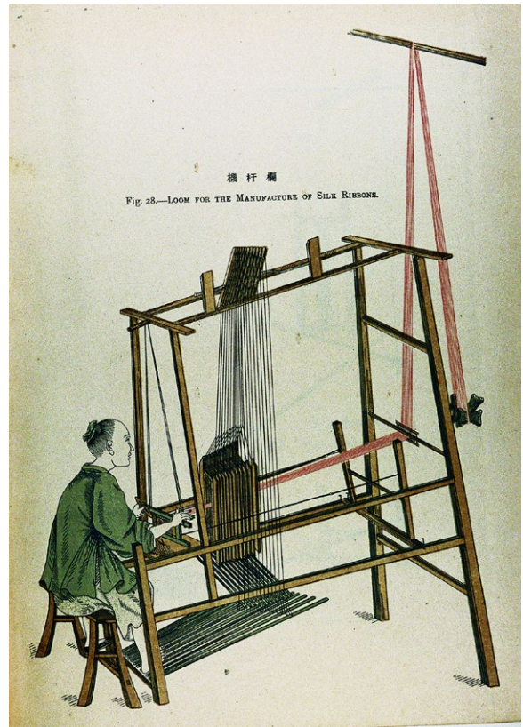
Fig 8. Multiple heddles and treadles loom in E. Rocher's report (after ZHAO 2005, p. 516).
