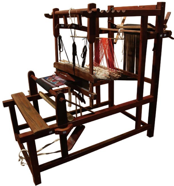
Fig 4. (left) Zhuang brocade loom from Jingxi in Guangxi Province; (right) Its multiple heddle pattern device.
