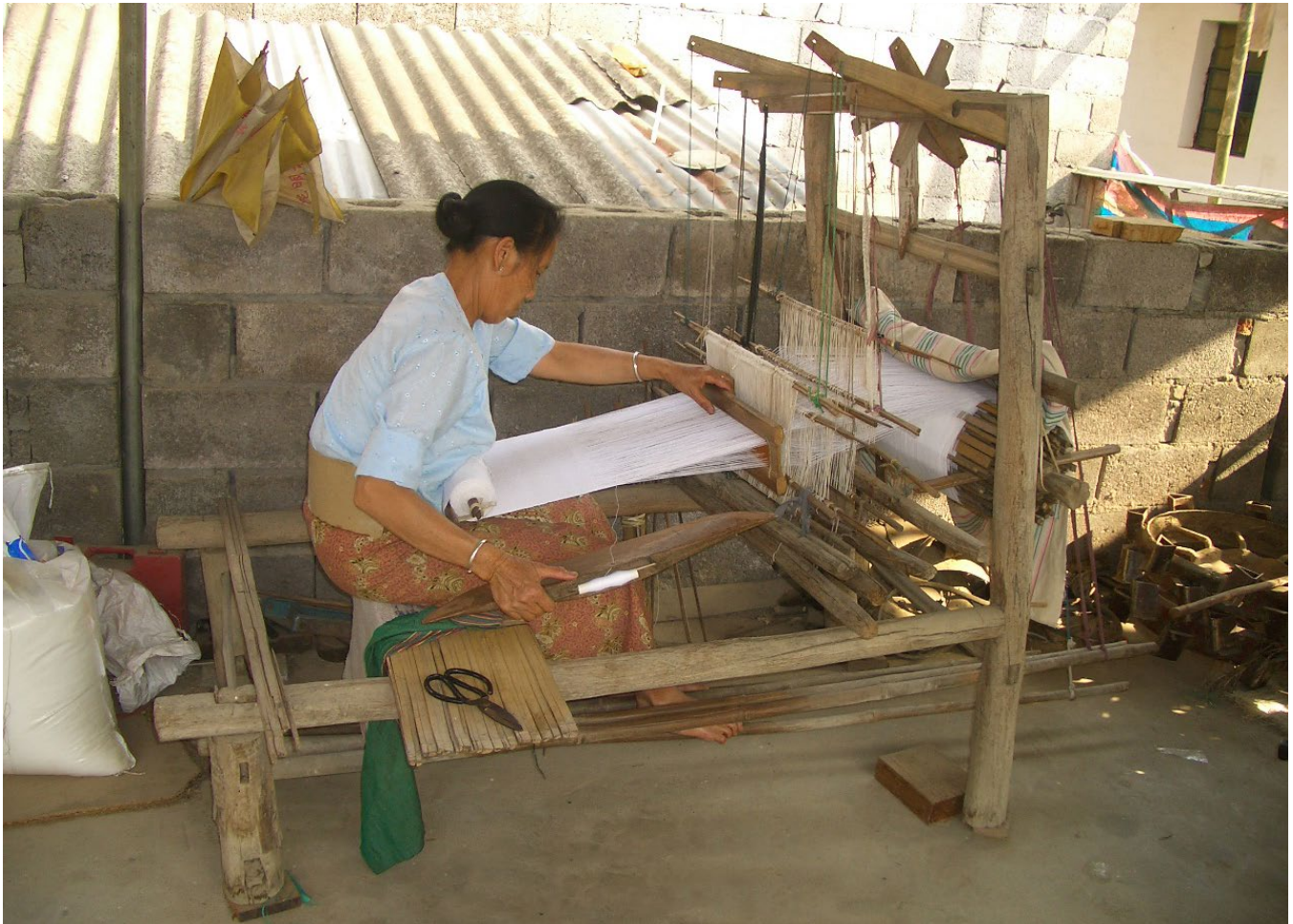
Fig 5b. Multiple heddles and treadles loom in the Dehong region, Yunnan Province.
