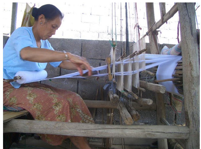
Fig 5a. Multiple heddles and treadles loom in the Dehong region, Yunnan Province.
