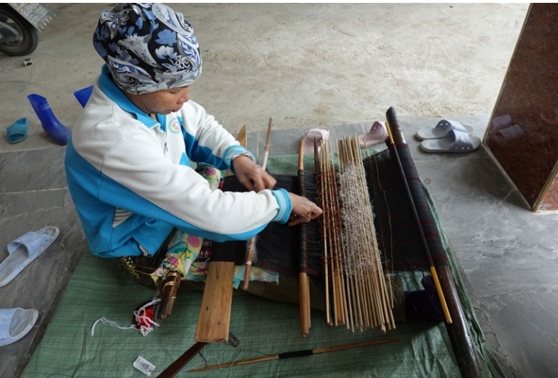
Fig 2. Li weaver using a backstrap loom with heddle-rod system, Hainan.
