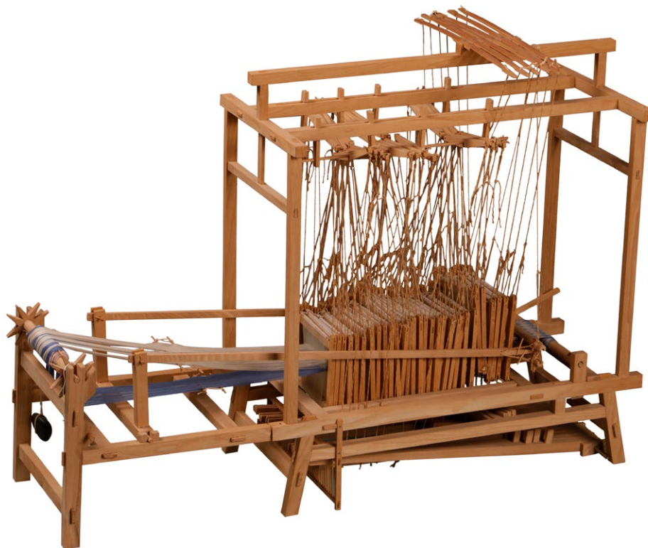
Fig 10. Model of the Multiple heddles and treadles loom from Shuangliu, Sichuan Province.
