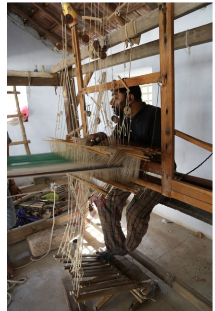
Fig 6. (left) Balanced multiple heddles and treadles loom of Bhujodi, Gujarat, India, on display at the China National Silk Museum, Hangzhou; (right) Weaver using the loom in Bhujodi.
