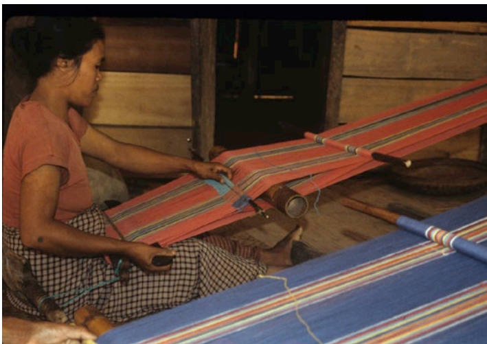
Fig 16. Woman weaving on a backstrap looms of I-type, with a heddle on a circular warp for weaving a warp-striped sarung . Bambang district (PUS), 1983/84. Image courtesy of G. Kenneth M.
