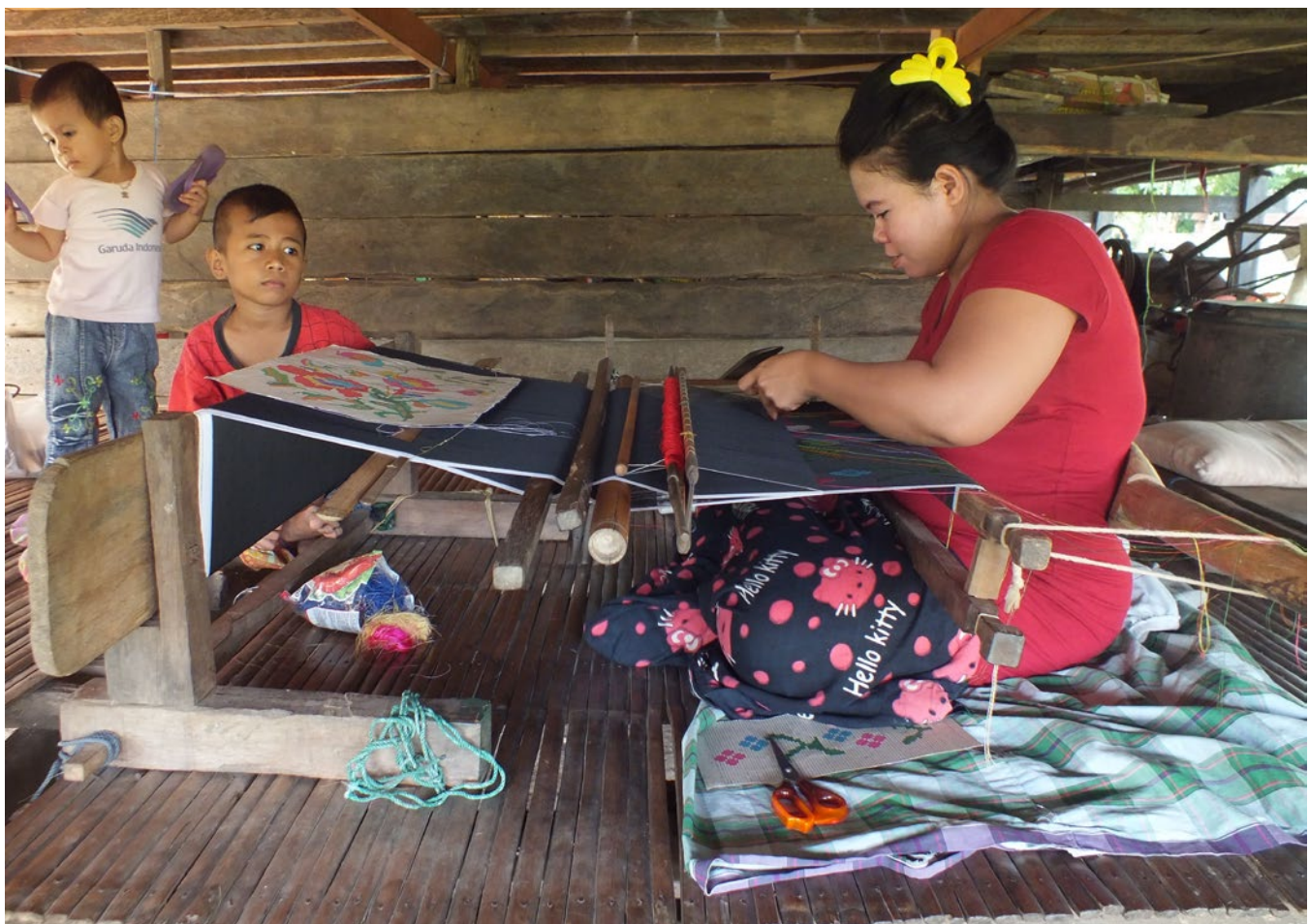
Fig 17. Woman weaving on a backstrap loom of II-type, with a heddle on a flat warp (as opposed to circular) that is passed through a reed. Sengkang district (Wajo Regency, South Sulawesi), 2017.
